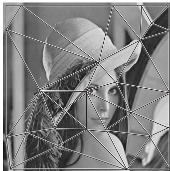
Figure 3.5: Example of image meshing [Lu and Hsu, 2005] for robust hashing. Each triangle of the mesh is then warped to a right-angled triangle and gives to a hash.
