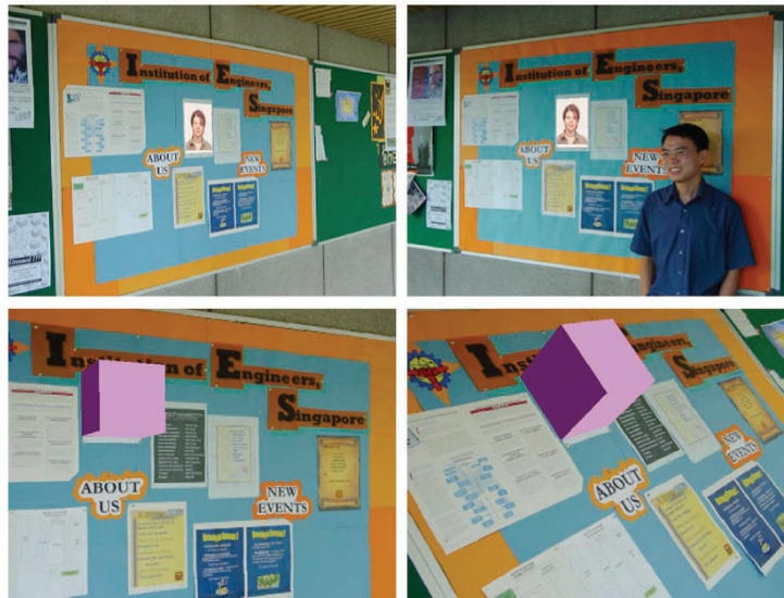
Figure 5.3: Pose computation from a reference plane image (taken from the real clipboard) and feature point frame-to-frame tracking [PXC02]. In the bottom row, the scene is augmented with a virtual 3D cube.
