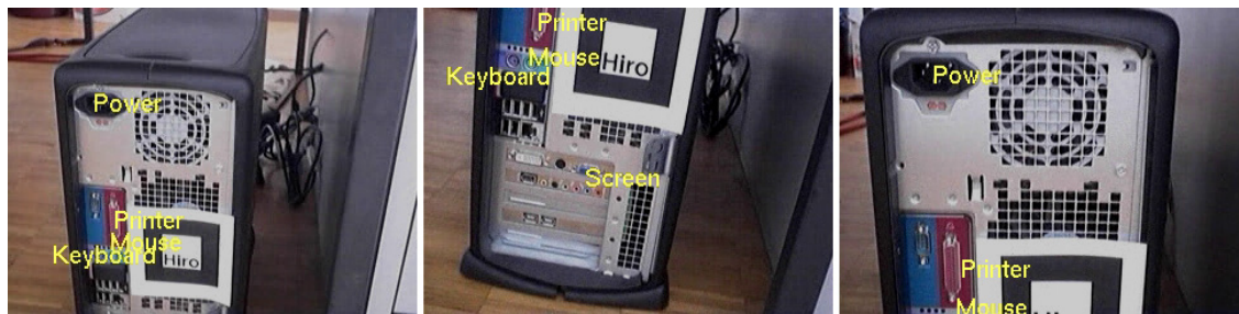
Figure 7.3: Machinery inspection assisted with augmented reality. The plugs of a Personal Computer are indicated. Augmented information is provided despite the occlusion of the marker.
