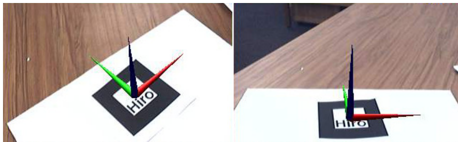
(b) Example of world coordinate overlaid on the marker for different real viewpoints.
