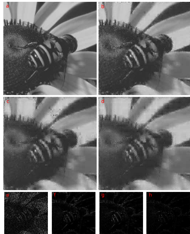
Figure 4. a: Truth. b: VB-Lap-tree . c: MAP-Lap-tree. d: VB-Lap-factor. e: \mathbf{y} (25%). f: \Delta(c, a) . g: \Delta(d, a) . h: \Delta(b, a) .
