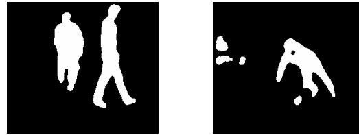
Figure 2. The result of background subtraction
