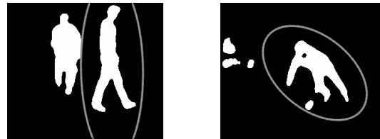
Figure 3. The result of elliptical approximation of an object
