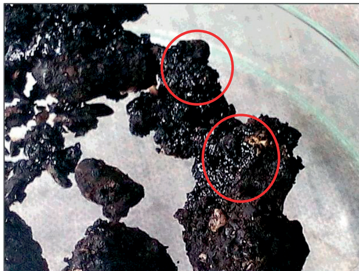
Figure 4.9 Part of RAP where crust was broken by abrasion effect of virgin aggregates.
