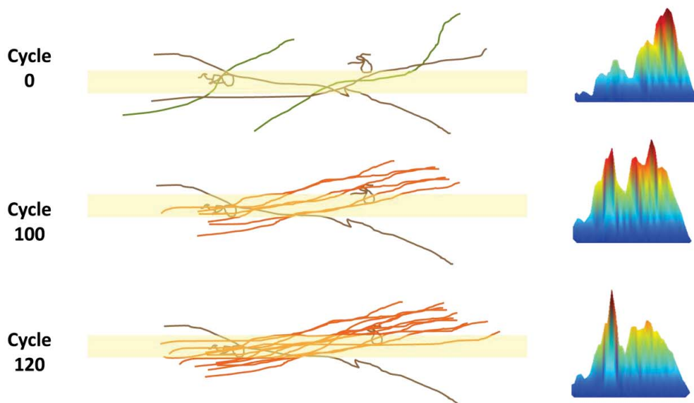
Figure 5.14 Illustration of the evolution of dislocation pile-up in region F (position 1)
