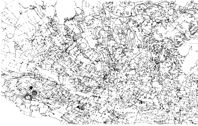
Fig. 5. The graph extracted from the geospatial data of OSM about an European city. The vertices and edges of the graph enables the representation of the geometrical shape of the roads.
