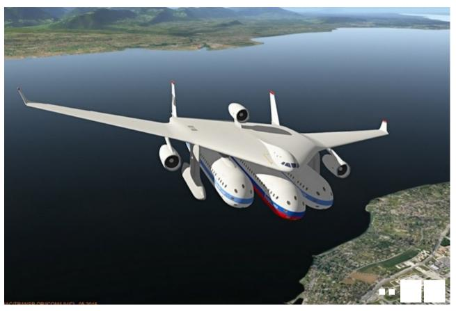
The modular Clip-Air concept, by which capsules would be transported by a fixed-wing aircraft. Courtesy the Ecole Polytechnique Fédérale de Lausanne (EPFL).
