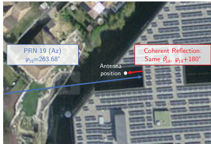
Figure 4.34 – Single specular reflection hypothesis to explain the main secondary peak in the DOA map for PRN 19.
