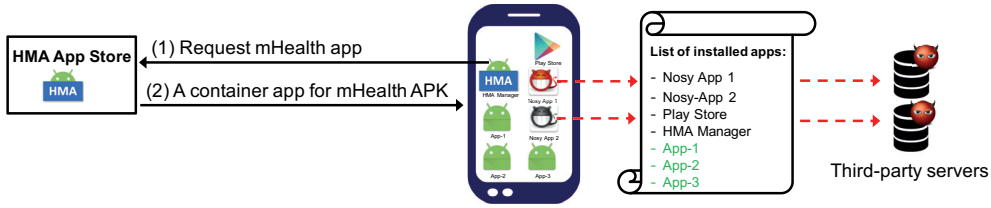
Figure 2.1: Overview of the HMA architecture. Nosy apps would only learn the generic names of the container apps.
