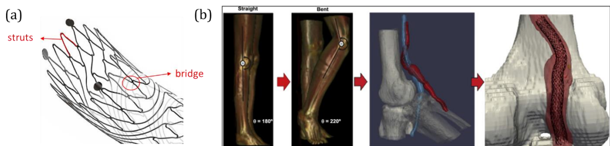
Figure 1.1 (a) The geometry of a NiTi stent consists of struts and bridges [9]. (b) The shape change of the NiTi stent in the artery near the knee [5].
