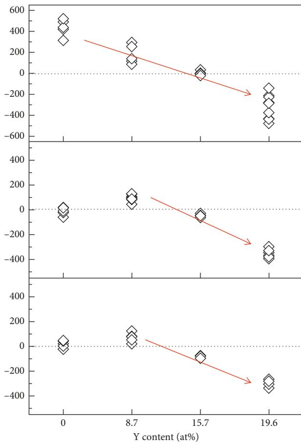
FIGURE 7: CuMn film TCR temperature dependence with various yttrium contents annealed at different temperatures.
