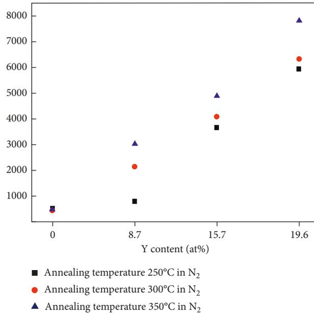
FIGURE 6: CuMn film room temperature resistivity with various yttrium contents annealed at different temperatures.
