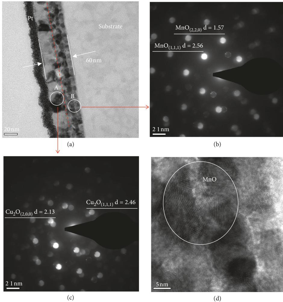
FIGURE 2: CuMn film TEM micrographs annealed at 350°C: (a) cross-section bright field, (b) selected-area electron diffraction at position A, (c) selected-area electron diffraction at position B, and (d) HRTEM micrographs at position B.
