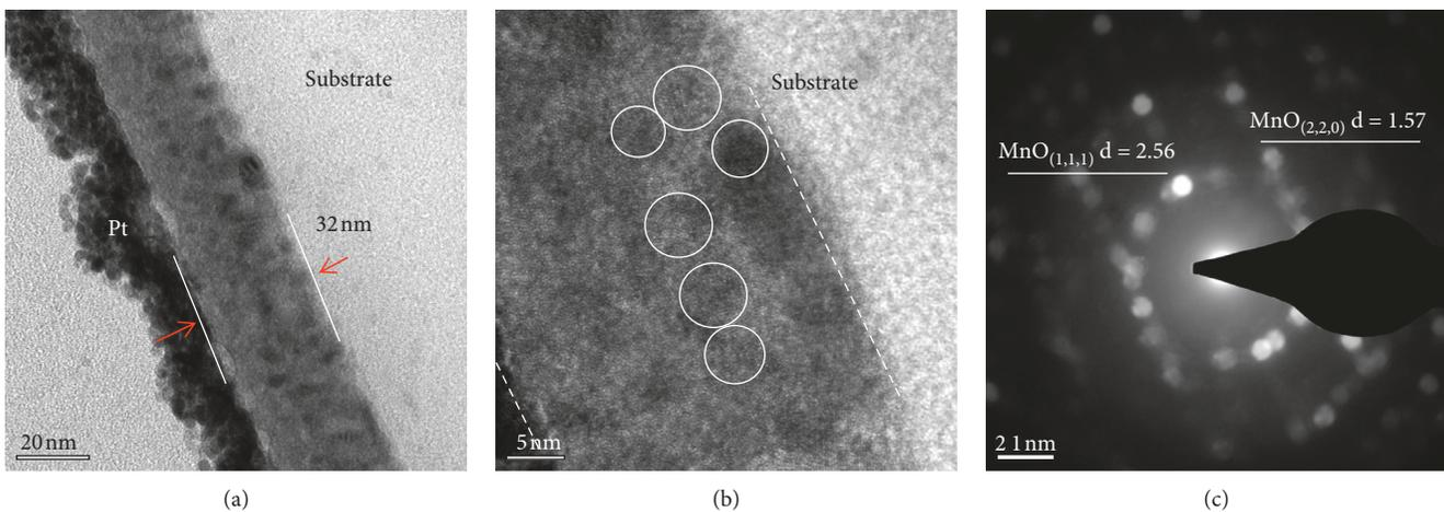
FIGURE 5: CuMn film TEM micrographs with 19.6 at.% Y addition annealed at 350°C: (a) cross-section bright field, (b) selected-area electron diffraction, (c) SAD analysis, and (d) HRTEM micrographs.
