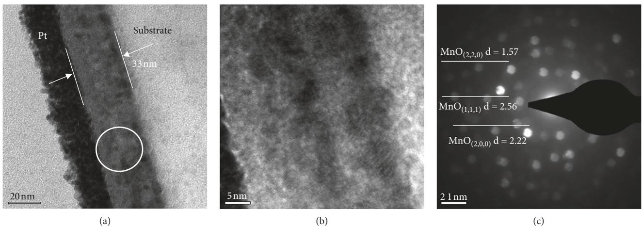
FIGURE 3: CuMn film TEM micrographs with 8.7 at.% Y addition annealed at 300°C: (a) cross-section bright field, (b) selected-area electron diffraction, (c) SAD analysis, and (d) HRTEM micrographs.
