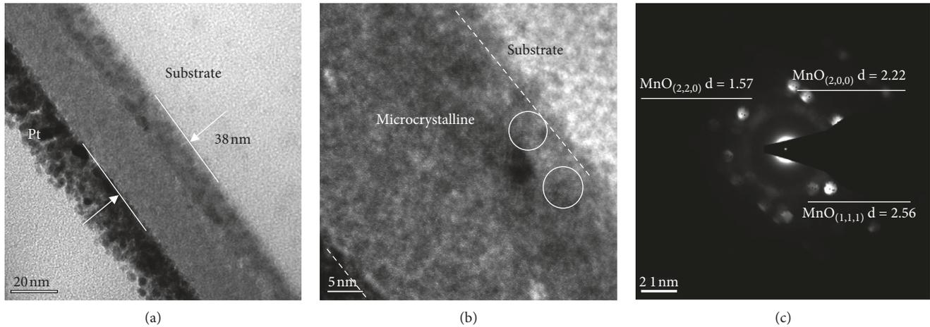
FIGURE 4: CuMn film TEM micrographs with 19.6 at.% Y addition annealed at 300°C: (a) cross-section bright field, (b) selected-area electron diffraction, (c) SAD analysis, and (d) HRTEM micrographs.
