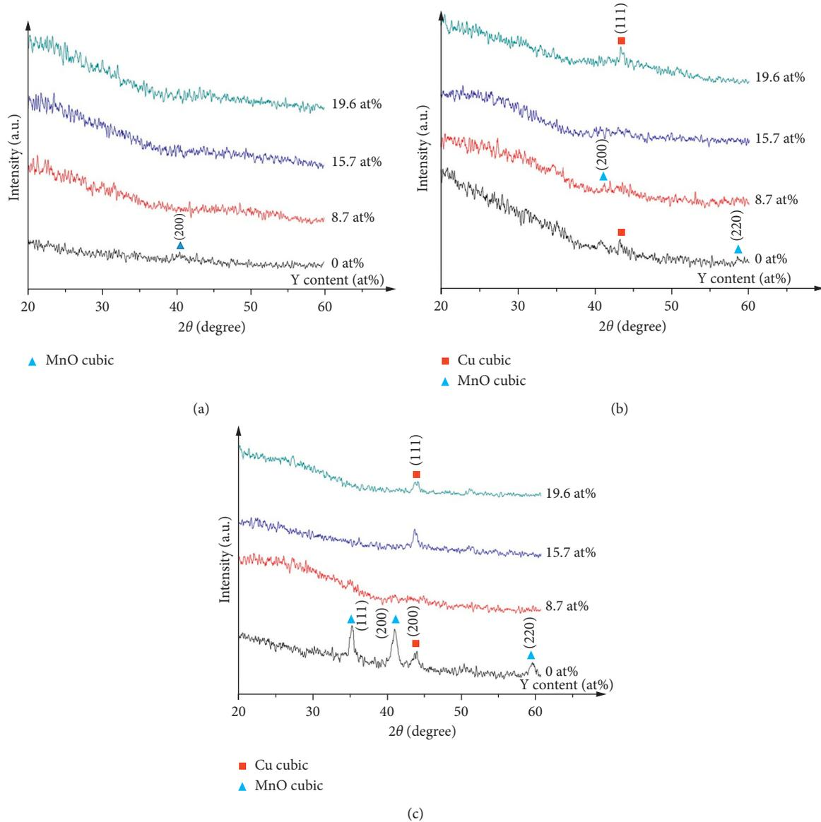
FIGURE 1: CuMnY thin-film X-ray diffraction patterns with various amounts of yttrium addition annealed at (a) 250°C, (b) 300°C, and (c) 350°C.
