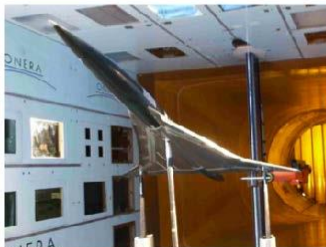
Figure 1: The EPISTLE model placed with the ONERA F1 wind tunnel
