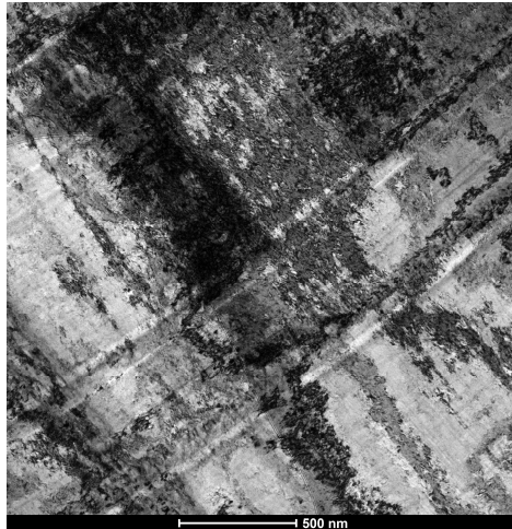
Figure 2-9 TEM BF image of red gold prepared by cryo-ultramicrotomy.
