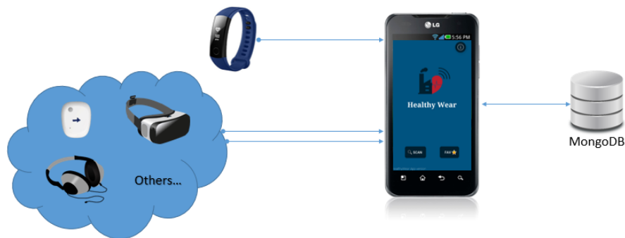
Figure 5. Overview of the applied wearable data flow.
