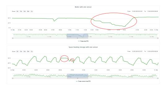
Figure 3.12 - Temperature of the boilers for DHW and SH in Lenzburg during the system failure
