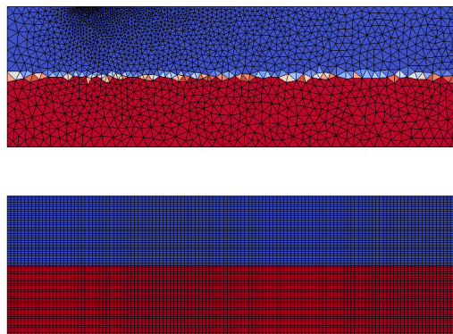
Figure 4.18 – Plunge pool scouring by an inclined impinging liquid jet. Intermediate mesh: finite elements (top), structured grid (bottom).
