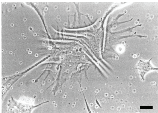
Figure 3.1 – Micrograph of wrinkles created by a fibroblast when plated on a silicone rubber substrate. Scalebar 10 \mu\text{m} . Taken from Harris et al. (1980)
