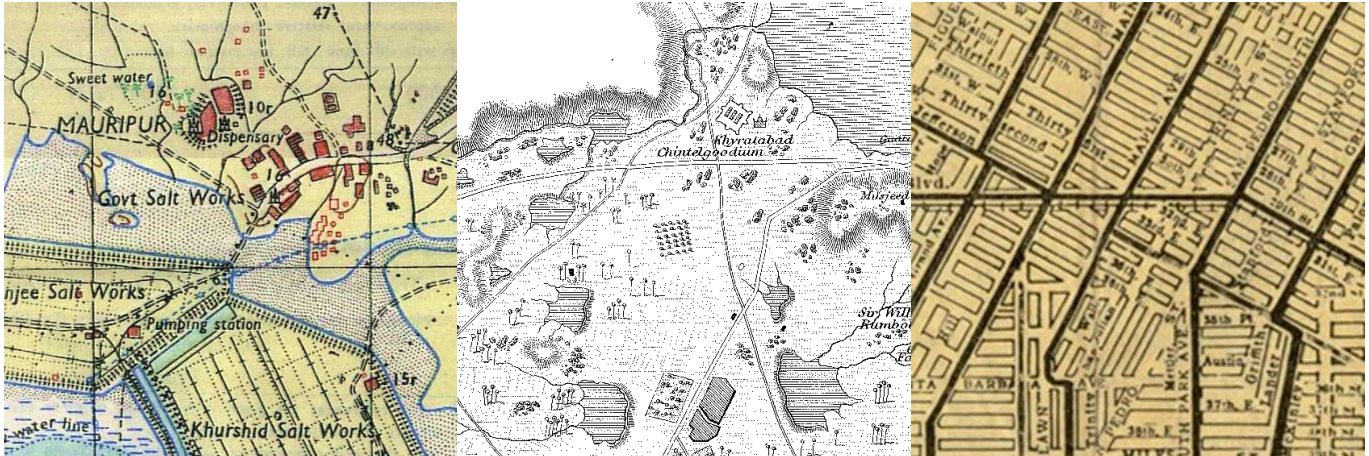
Figure 2.3.11 Digitization imperfections. From left to right: 1) poor color scanning quality and brightness jumps [99]; 2) loss of information due to image binarization [100]; 3) low resolution [101].
