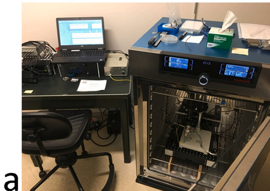
Fig. 3. E. coli nanomotion was measured at 23 °C and at 30 °C inside a temperature-controlled incubator. a. The NMD device was operated inside the Peltier temperature-controlled incubator together with a vibration isolation table and digital microscope. b. E. coli cell nanomotion was measured at 23 °C for 2 h in LB medium prior to exchange LB with isotonic buffer for two hours (PBS: no carbon source), this was then followed by inactivation with glutaraldehyde (PBS-Dead) for one hour. The boxes defined by 25th and 75th quartiles (outliers shown in red), represent 1-hour data bins. c. E. coli cells analyzed at 30 °C in LB, PBS and after inactivation with glutaraldehyde (PBS-Dead). Plot representation is the same as in (b). Given variability between different cantilevers and cell loads, the data in b and c are not comparable. (For interpretation of the references to color in this figure legend, the reader is referred to the web version of this article.)
