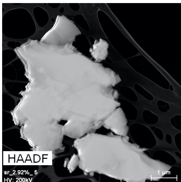
Figure 3.3 – HAADF-STEM image of a 2.92% Sr-doped \beta -TCP powder, thermally treated for XRD.
