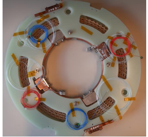
Fig. 2. The small SFCL pancake prototype comprising two conductors (1 and 2) in a bi-filar winding co-wound with three optical fibres on each conductor. There are five turns per conductor with insulating spacer between turns visible in the photo. One optical fibre on each conductor is spliced on both ends of each conductor (the external end fibres visible in blue and internal end spliced fibres visible in red, for each conductor)
