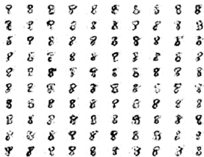
Figure 11: Generated samples from a GAN exhibiting mode collapse and only creating the digit 8.
