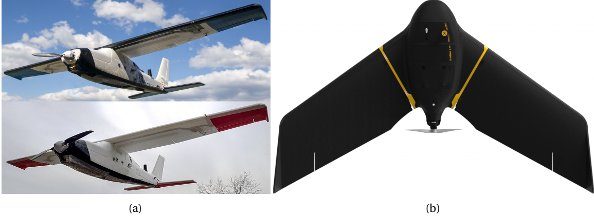
Figure 6.1: Fixed-wing platform with 5 control surfaces (left): the two versions of the TOPOplane (a) version-1 (top) and version-2 (bottom), and the eBeeX from senseFly (b)
