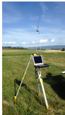
Figure 6.6: Ground Control Station set up with the operator's computer running QGC and the telemetry transceiver
