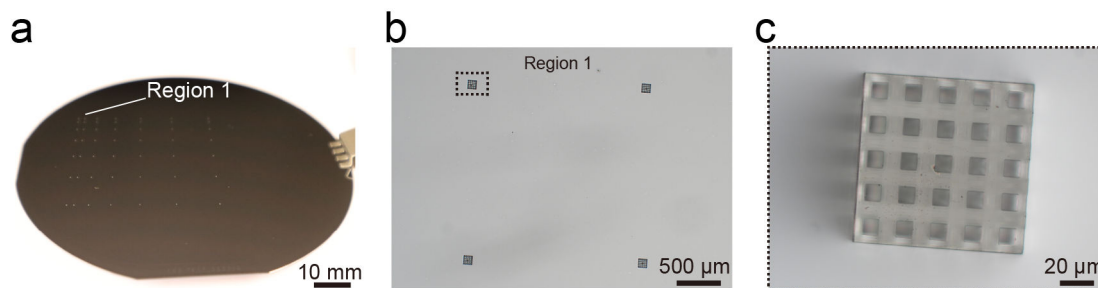
Figure 4.10: Transfer result of the microsccaffold array. (a). Simple sketch showing the distribution of the 49 microscavolds on the receiver after transfer. In vertical and horizontal directions, the pitch distance varies from 2000 to 12000 \mu\text{m} . (b). Optical image of the 4-inch receiver with all the 49 transferred microscavolds, forming a 7 \times 7 array with varying pitch distance. (c). High-magnification image of Region 1. A 2 \times 2 scaffold array is displayed in this image with a pitch distance of 2000 \mu\text{m} . (d). High-magnification image of 1 scaffold in (c).
