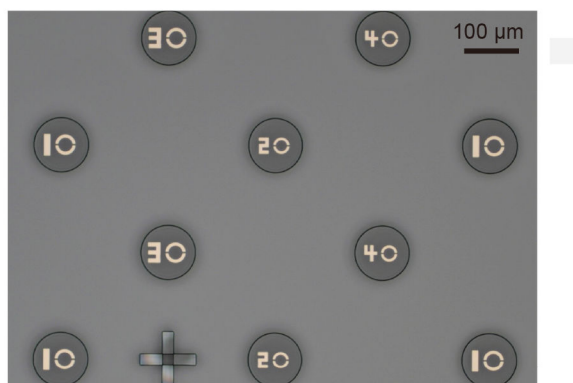
Figure A.1: Metal number patterned SU-8 microdisk. Ten SU-8 microdisks are shown in the image. Metal numbers (Cr/Au, 5/50 nm) "10", "20", "30", and "40" are patterned on top of the SU-8 microdisks by stencil lithography.
