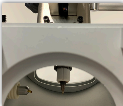
Figure 6.6. ESI source with a syringe pump used in this work.
