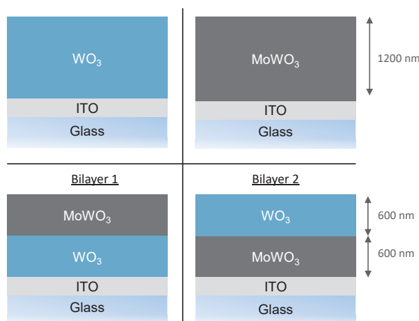
Figure 6.10: Cross-section schematic of the four combinations chosen to study the propagation of lithium in the material. The two configurations on the upper half are used as reference and the two at the bottom are the investigated bilayers.
