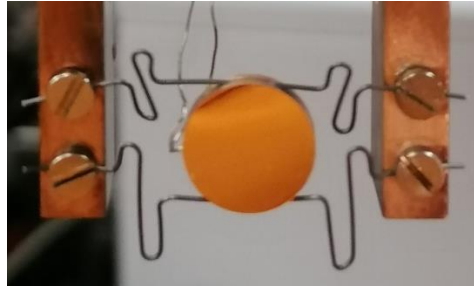
Fig. 2.7: A Cu(111) surface held in between two tungsten wires, used for surface heating and cooling.
