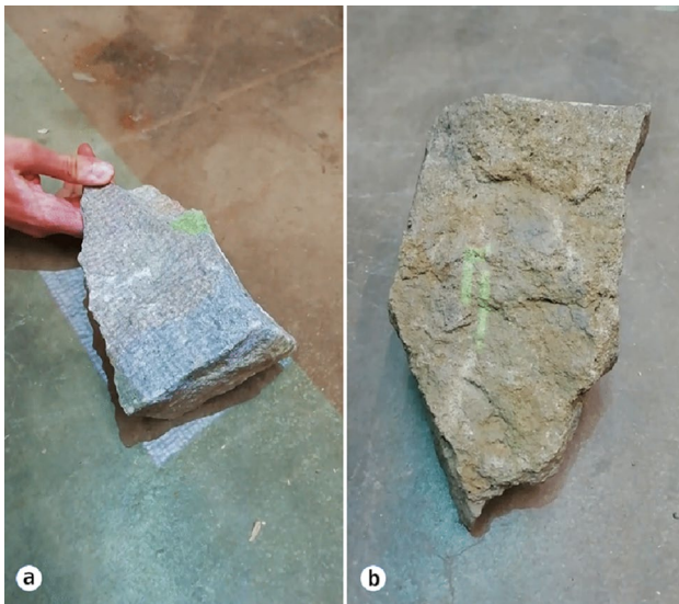
Fig. 10 Preliminary tests for the developing of an efficient projected mapping interface: (a) overload of projected information, (b) insufficient highlighted pixels to effectively display instructions
