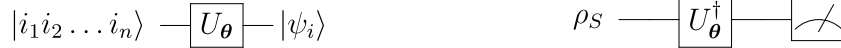
Figure 9. We summarize the circuits used to evaluate the cost function for the CCPS ansatz. (Left) A generic way to prepare a randomly sampled eigenvector of the CCPS state. Here, the state |i_1 i_2 \dots i_n\rangle is a short-hand for an n qubit computational basis state, so each i_j is either 0 or 1. Given the randomly sampled bitstring, we can prepare the desired state with single qubit X gates, and then we apply the same unitary U_\theta regardless of the randomly sampled input. (Right) Here, we provide a circuit to sample the distribution q_\theta(i) defined in equation (B14). We simply prepare \rho_S , apply U_\theta^\dagger , and measure each qubit separately in the computational basis. By equation (B14) and the fact that p_\phi(i) is stored classically, we can therefore compute the desired cross term using a classical SWAP test as described in the main text around equation (24).
