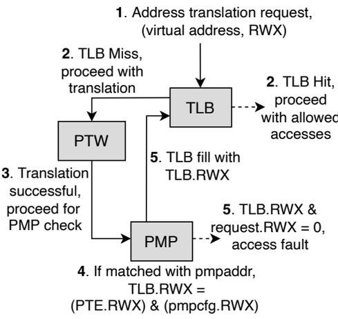
(b) Address translation process. & indicates logical AND operation. Dashed lines indicate alternative steps.
