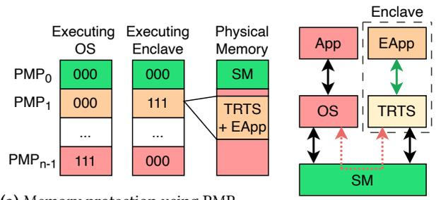
(a) Memory protection using PMP. PMP entries show pmpcfg.RWX bit values. (b) Mode switches.
