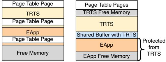
**Figure 6.** Enclave memory layout in Keystone (left) and Keystone-LP (right).
