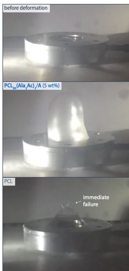
Figure 36. Facilitated film blowing. Film blowing experiment at 70 °C, demonstrating that, upon application of an overpressure of 0.1 bar, sheets (prepared by hot-pressing at 80 °C and cooling to room temperature at a rate of 10 °C/min) from PCL 80 (Ala 2 Ac) 2 /A (5 wt%) form stable bubbles with a uniform materials distribution up to substantial deformations, which is not possible with either PCL 80 /A blends or pristine PCL.
