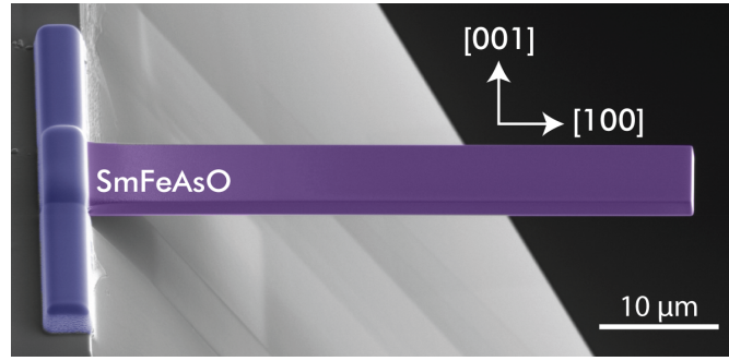
Figure 6.4: SEM image of a FIB-fabricated cantilever of SmFeAsO.
