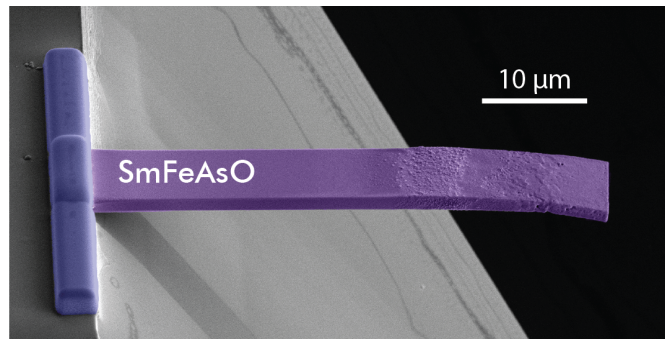
Figure 5.9: SEM image of a SmFeAsO cantilever damaged from laser heating during measurement.
