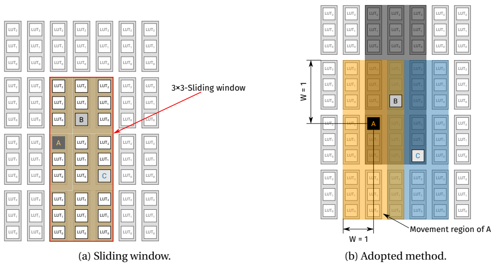
Figure 8.11: Movement freedom of movable nodes. Figure 8.11a shows a portion of the FPGA with a sliding window of 3 \times 3 clusters used to select movable nodes. Inside this window, all nodes are movable and each of them can be placed anywhere in the window. Figure 8.11b shows the approach we take in this chapter. Only a subset of nodes in each square region of the FPGA is selected for movement. Each of them can be placed at any position inside a square of half-width W , centered at its original cluster.
