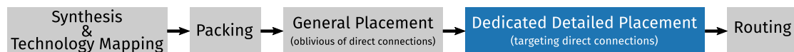
Figure 8.3: Position of the proposed detailed placement algorithm in a typical FPGA CAD flow.
