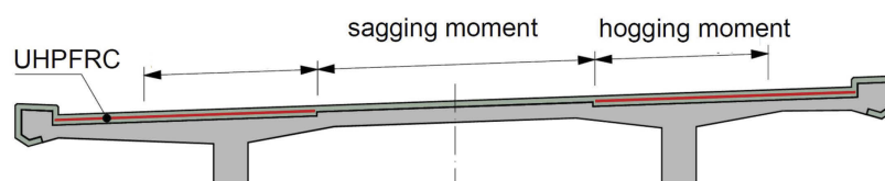
Figure 5. Concept of increasing the resistance of the original RC deck slab by means of the R-UHPFRC layer forming a strong R-UHPFRC tension chord in the hogging moment zone.
