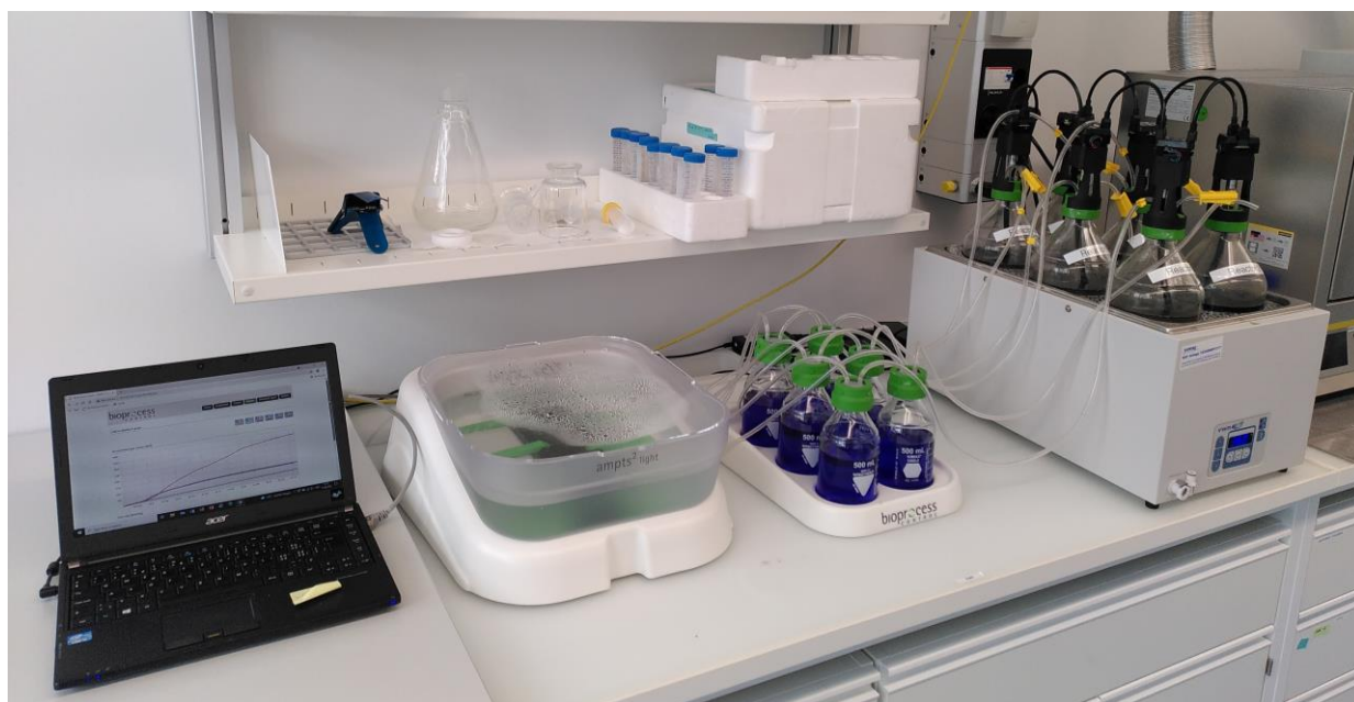
Figure 6 - AMPTS II Light device (from right to left: the sample incubation unit, the \text{CO}_2 -absorbing unit, and the gas volume measuring device)
