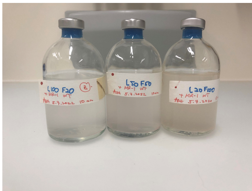
Figure D.1: Samples of different Lactate:Fumarate ratios after 48 hours growth, where pink color was obtained for fumarate limited system. Note that for the sample Lactate 100 mM: Fumarate 20 mM, this color is less intense due to the lower biomass produced compared to the other two cases.
