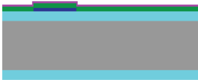
Fig. 6. Cross section after the AlScN and Al deposition. In dark blue the seeding layer + Pt, in light blue the SiN, in green the AlScN, in purple the Al and in gray the Si.
