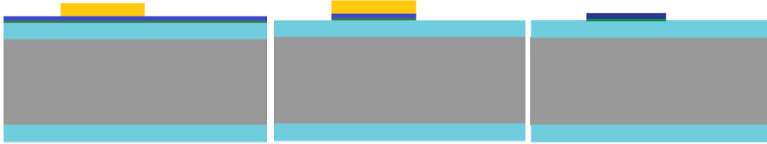
Fig. 5. Cross section before (left) and after (middle and right) ion beam etching. In dark blue the Pt, in light blue the SiN, in green Ti or AlN, in yellow the photoresist (AZ ECI 3007 or AZ 10XT-07) and in gray the Si.
