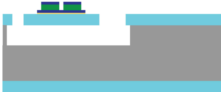
Fig. 1. Typical cross section of one device. In dark blue the Pt, in yellow the Ti, in gray the Si, in light blue the SiN and in green the AlScN. Dimensions are not in scale.
