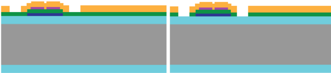
Fig. 10. Cross section before (left) and after (right) ion beam etching. In dark blue the seeding layer + Pt, in light blue the SiN, in green the AlScN, in yellow the resist, in purple the Al and in gray the Si.
