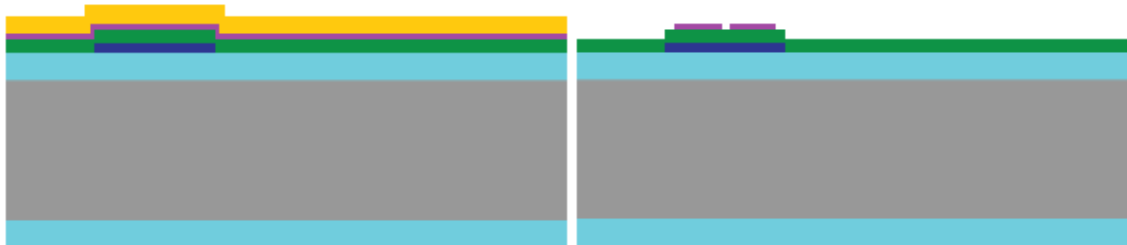
Fig. 7. Cross section before (left) and after (right) resist development. In dark blue the seeding layer + Pt, in light blue the SiN, in green the AlScN, in yellow the photoresist (AZ 10XT-07), in purple the Al and in gray the Si.
