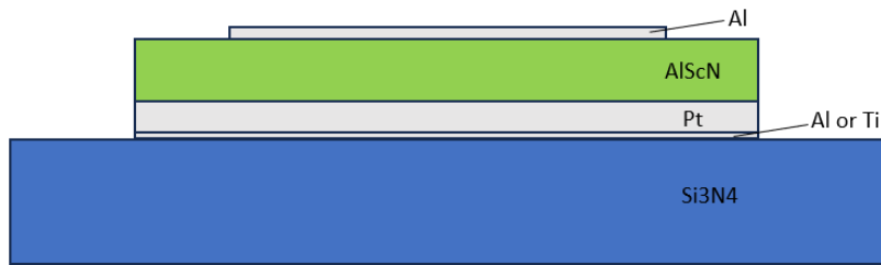
Figure 1: Cross-section view of the design of the singly-clamped devices
