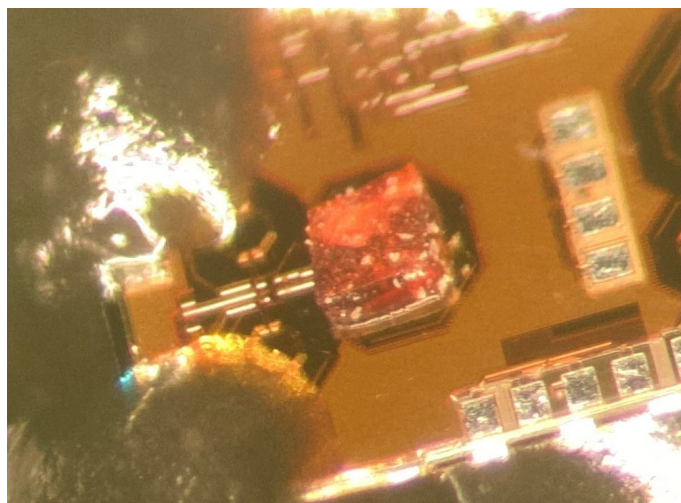
Figure 2.10: Picture of the chip together with the 2%BDPA:SEBS sample placed on top of the concentric ESR and NMR microcoils.
