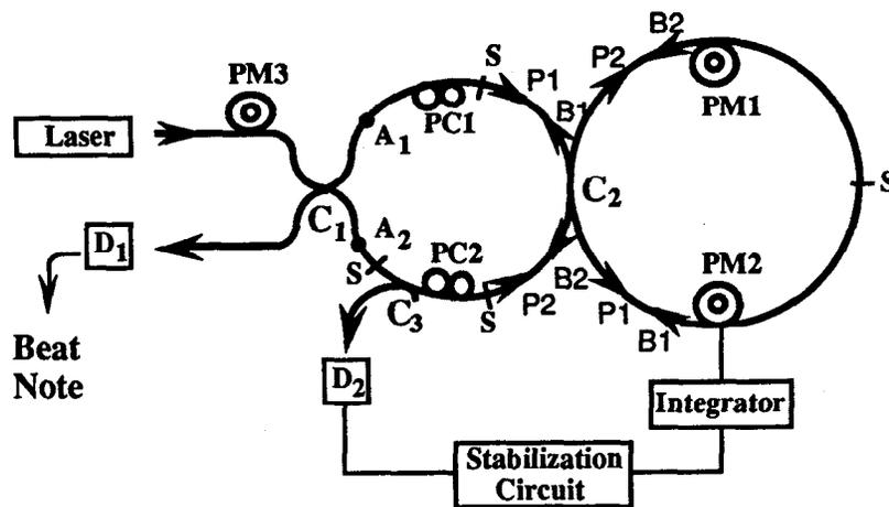
Figure 1. Schematic diagram of the BFOG system: P1 and P2, pump waves; B1 and B2 Brillouin waves.
