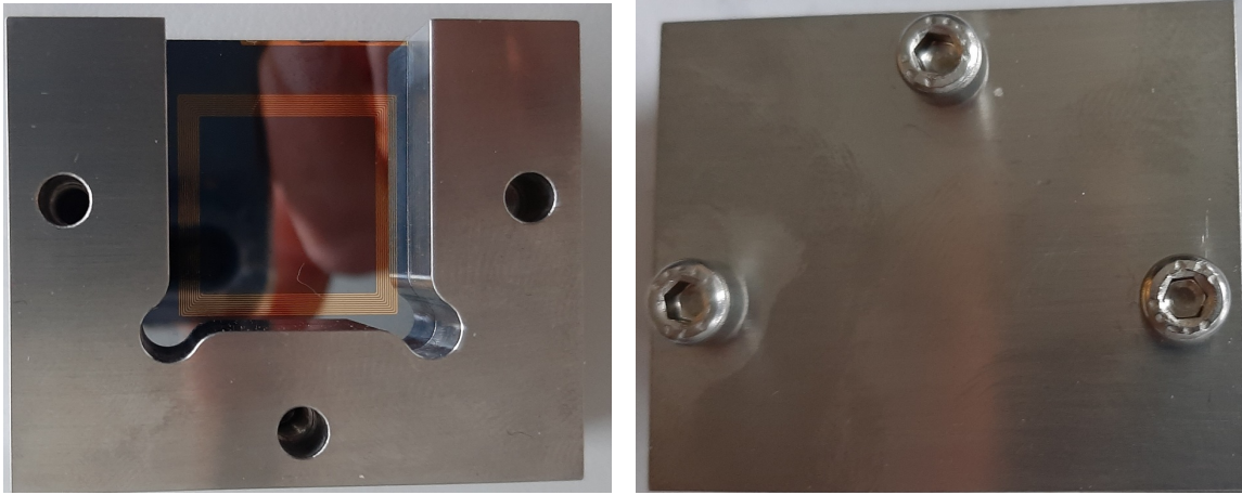
Figure 7. The sensor-assembly prototype, on the left without cover so as to show the circuits, on the right with the cover and the three guiding M4 pins. One of the sides of the holder is open to allow for the mounting of the ICB connector to the in-vessel cabling, which is currently being prototyped.
