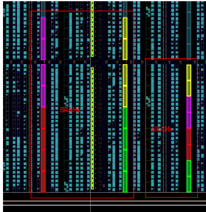
Figure 4.10 – Enforcing relative placement of BRAMs and URAMs in cores. We show the register files and instruction/data memories of four cores. Cells with the same color belong to the same core. BRAMs are enforced to be placed in always the same order (RS1, RS2, RS3, RS4; from top to bottom). A similar strategy is used to enforce that the instruction memory always appear above the data memory (this is less necessary, but we found it leads to more regular local floorplans if enforced).
