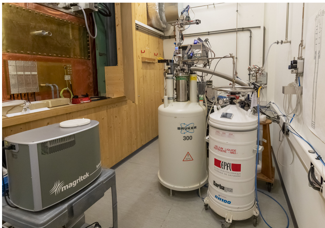
Figure 4.1: Picture of the dDNP setup upgraded in this chapter. The 5T/1.15K DNP polarizer is composed of a liquid-helium VTI inserted into a wide-bore NMR magnet ramped up to a magnetic field strength of 5 T. All vacuum pumps are installed behind the polarizer. Liquid helium is drawn from an external 100 L storage tank. Part of the liquid-state polarization measurements are performed in the benchtop ^1\text{H}/^{19}\text{F}/^{13}\text{C}/^{129}\text{Xe} 1.05 T (44.77 MHz ^1\text{H} frequency) NMR spectrometer in the foreground, while the remaining experiments are performed in the 14.1T MRI scanner located behind the filter panel.
