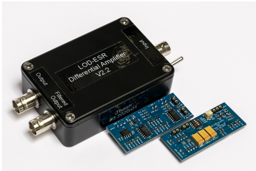
Figure A.4: Pictures of the LOD-ESR differential amplifier enclosure, and both sides of the assembled printed circuit board.
