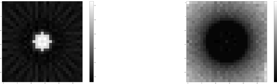
Figure 4.6: Left : MAP reconstruction estimation performed with Conjugate Gradient, with a least square data-fidelity term. Right : Pixel-wise uncertainty quantification using the method presented above.
