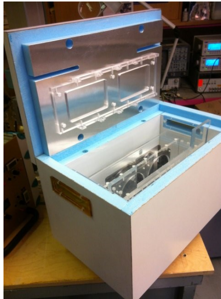
Figure 4.8: A photograph of the cold box with the cooling elements. The samples that are going under irradiation are attached to the lid of the cold box. The cold box contains a special opening for the insertion of the pre-calibrated gas mixture to avoid having condensation inside when operating at negative temperatures.
