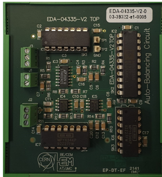
Figure 5.6: Single channel PCB prototype for capacitive humidity sensor readout.
