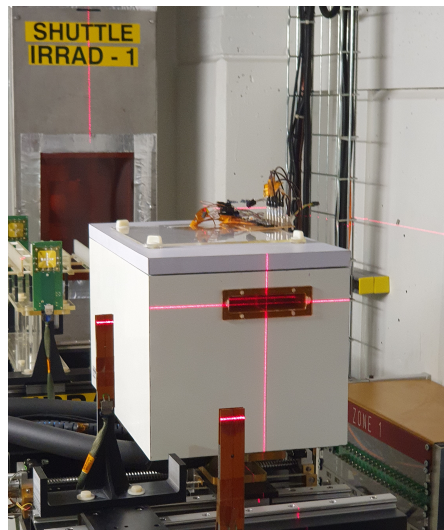
Figure 4.10: A photograph of the cold box with the samples inside positioned on one of the tables in the radiation area. The lasers show the center of the incoming proton beam.
