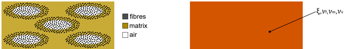
Figure 1.12: Schematical representation of the thermoplastic composite at the meso scale on the left, and the corresponding homogenized medium with descriptors on the right: the impregnation degree \xi , the fibre volume content \nu_f , the matrix volume content \nu_m and the void volume content \nu_v .
