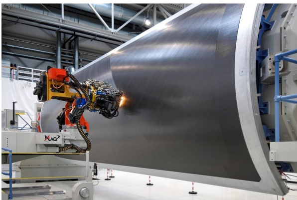
Figure 1.4: Picture of the automated tape laying process for the production of the upper shell fuselage skin section of an Airbus A350. A robotic arm continuously heats, places and consolidates layers of tapes to produce the desired geometry. While ATL is currently mostly used with thermoset composites, recent progress enables its application to thermoplastic composites as showcased in Figure 1.5.
