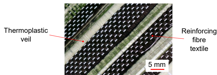
Figure 5.1: Picture of a hybrid side-by-side textile based on quasi-unidirectional carbon fibres and polyetherimide veils [156]. The textile stack has a partial and staggered cutaway, unveiling the different layers of the stack.
