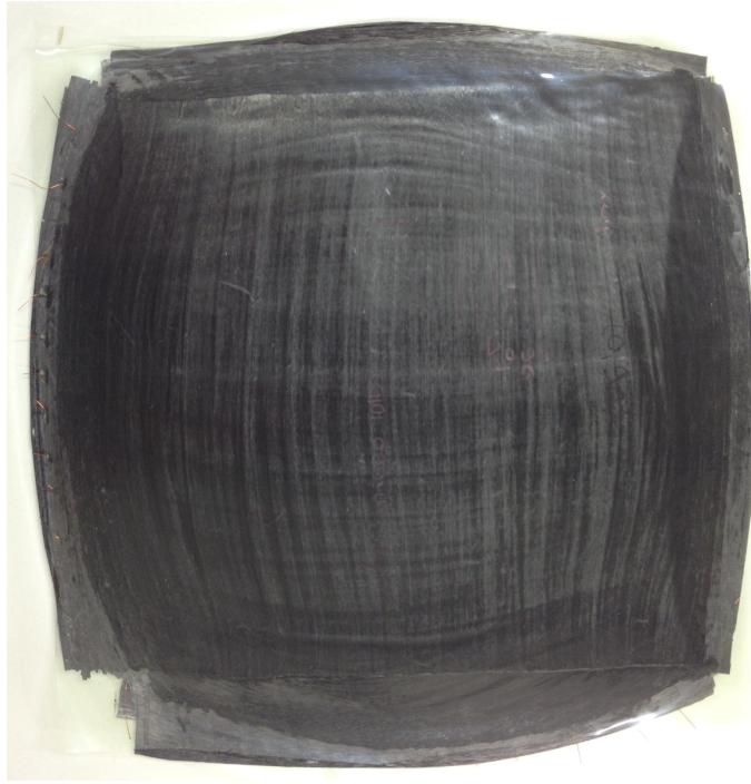
Figure 2.10: Photograph of a [0/90]_6 stack of UD layers after compression, where one can clearly see fibre displacement and waviness [108].
