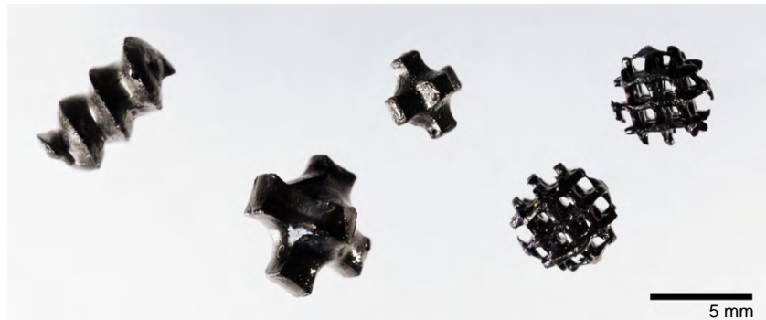
Figure 6.7: Examples of printed silicon oxycarbide ceramic components ; including a screw with an open axial channel, two three-dimensional crosses, and two spherical woodpiles.
