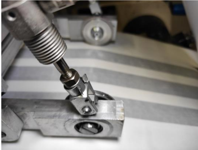
Figure 4.2 Trimming to final dimensions of the tow-by-tow carbon-glass thin ply prepreg.
