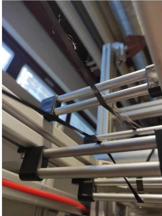
Figure 4.6 Fiber break of a tow of carbon fiber due to friction between the filaments and the static aluminum spreading bars of the mechanical pre-spreading stage.
