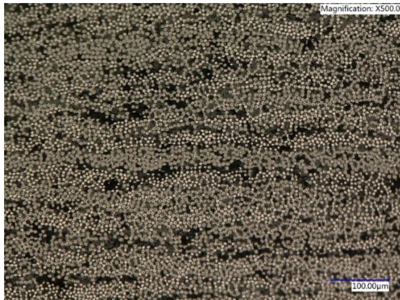
Figure 3.5 In the case of unidirectional (UD) fiber-reinforced composites, the microstructure corresponds to the fibers cross-section distribution. A typical microstructural profile of a laminate manufactured with 34-700 thin-ply prepreg.
