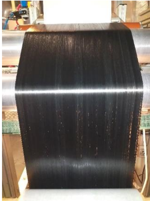
Figure 5.9 Carbon (HR40) – carbon (34-700) tow-level thin-ply hybrids tow-by tow Test 1: ^{31}T^{90} .
