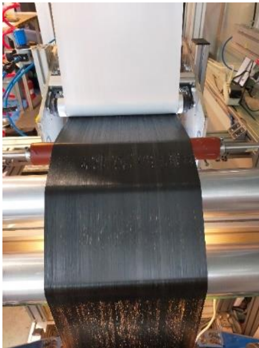
Figure 5.11 Carbon (HR40) – carbon (34-700) tow-level thin-ply hybrids tow-by-tow Test 3: 31 T 45 .
