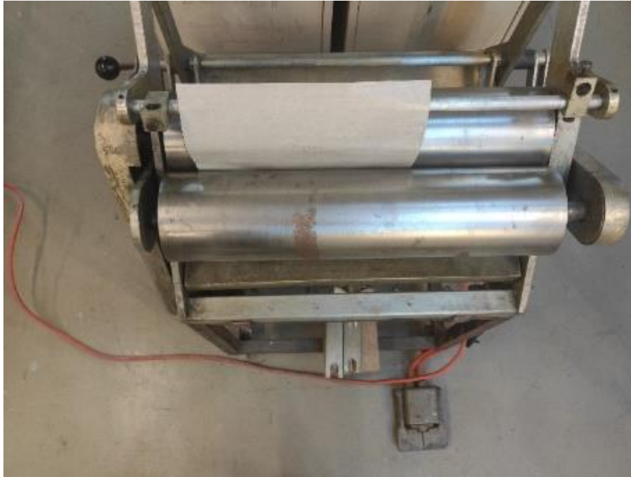
Figure 6.13 Calendering apparatus Wessex Resin and Adhesives Ltd. (Made in England) prepreg that was modified to be used as a calendering apparatus.
