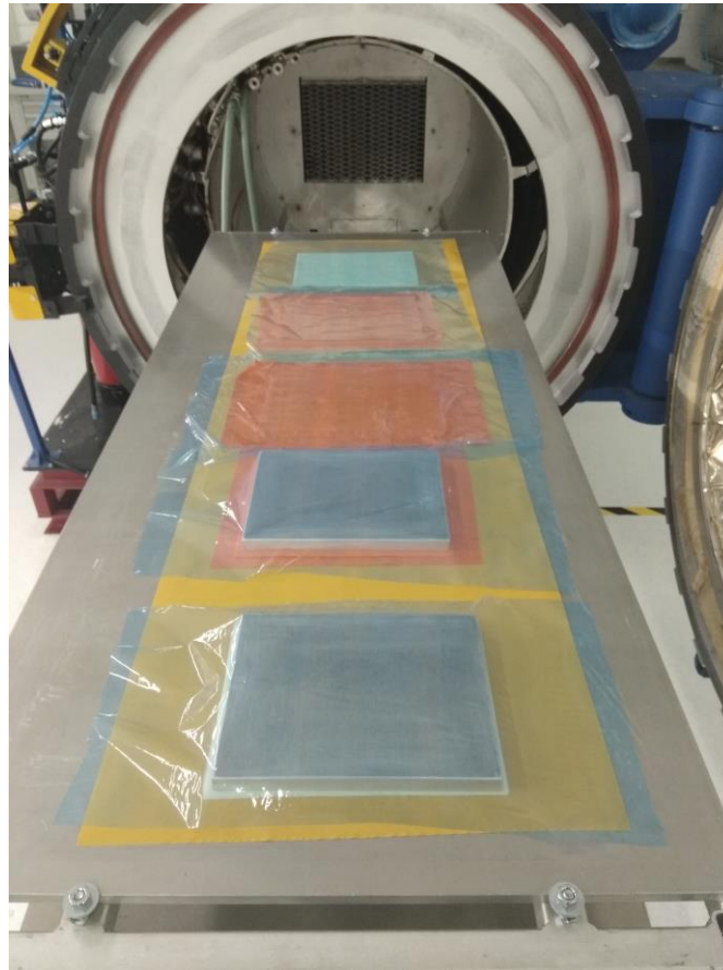
Figure 3.3 Curing multiple laminates with different curing set-ups to define the best-performing one.
