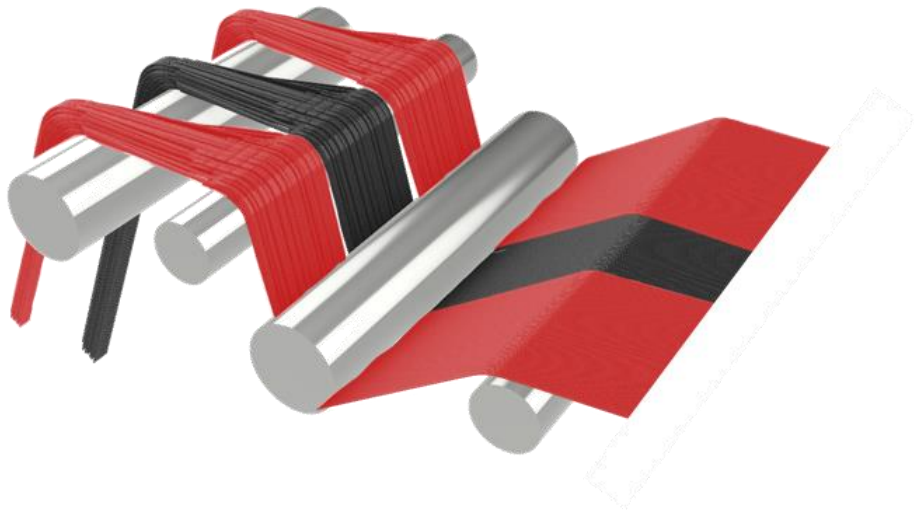
Figure 5.5 Schematic of simultaneous spreading of two dissimilar fibers in a tow-by-tow hybrid configuration.
