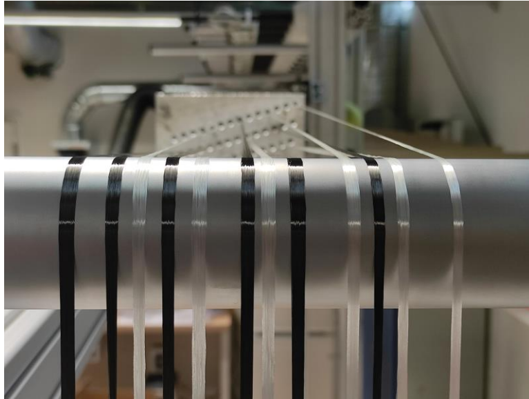
Figure 5.7 Tow of carbon and glass fibers arranged side by side before entering the main tow spreading of the prepreg process.
