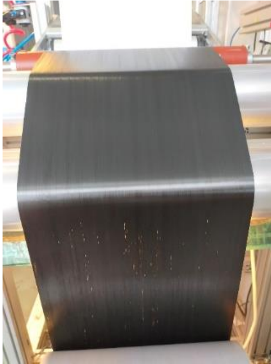
Figure 5.10 Carbon (HR40) – carbon (34-700) tow-level thin-ply hybrids tow-by-tow Test 2: 25 T 90 .
