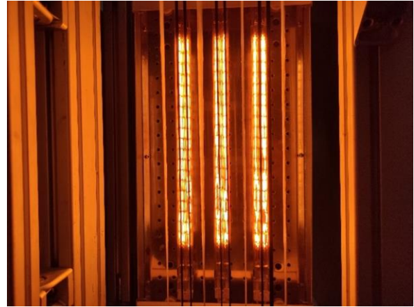
Figure 4.10 Thermal treatment stage a) Schematic of fiber coating removal stage b) fiber tows inside the thermal treatment chamber.
