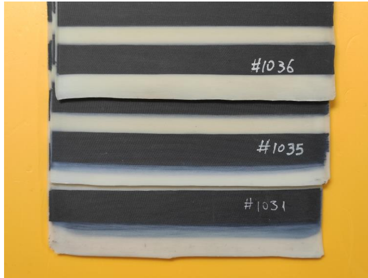
Figure 7.4 Reduction of the barrelling effect with optimized curing methods that reduced the in-plane movement of the fibrous network to neighboring tows.
