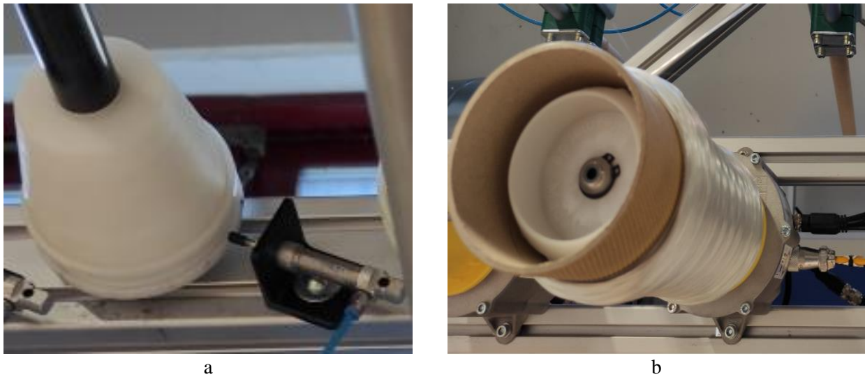
Figure 5.3 a) custom-made pneumatic unwinding unit, b) electronically controlled unwinding unit (EGA).
