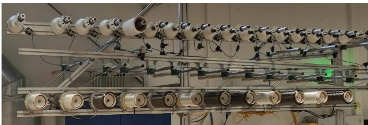
Figure 5.2 Photograph of the experimental setup to illustrate the fiber creels of a creel stand and show two different types of unwinding units.
