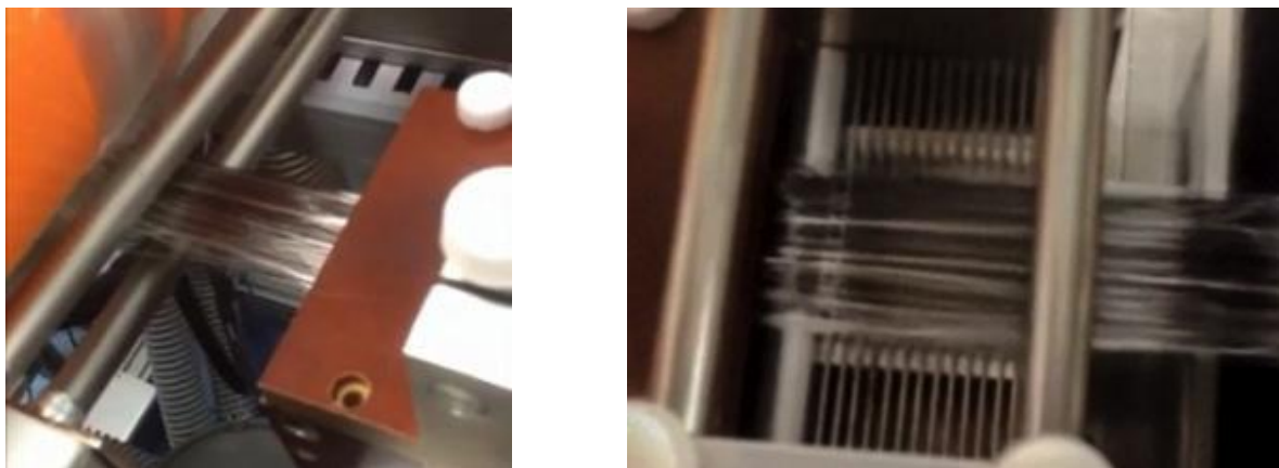
a b Figure 2.16 Parts of the air-assisted where the co-mingling of the carbon fiber (CF) and glass fibers (GF) appearance of the combined GF/GF tows. (a) before entering (b) during commingling process inside the spreading unit [83].
