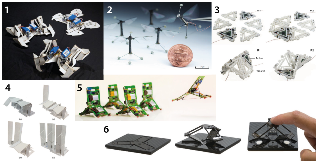
Figure 1.2: Origami robots take advantage of folding patterns for enhanced manufacturing processes, functional capabilities and adaptive characteristics. 1. Felton et al. (2014) [29] developed a method to build self-folding machines. 2. Ma et al. (2013) [39] achieved the first controlled flight of a biologically-inspired, insect-scale robot, the Robobee. 3. Belke et al. (2017) [27] take advantage of origami folding patterns to create a modular origami (MORI) robot system made of triangularly shaped modules allowing them to fold among themselves. 4. Zuliani et al. (2018) [25] use the folded structures to transform the configuration of a set of fingers using a minimal actuation. 5. Zhakypov et al. [31] developed the Tribot, a multi-locomotion scalable milli-robots biologically-inspired. 6. Mintchev et al. [40] took advantage of the origami structure to create foldable and interactive fingertip devices.
