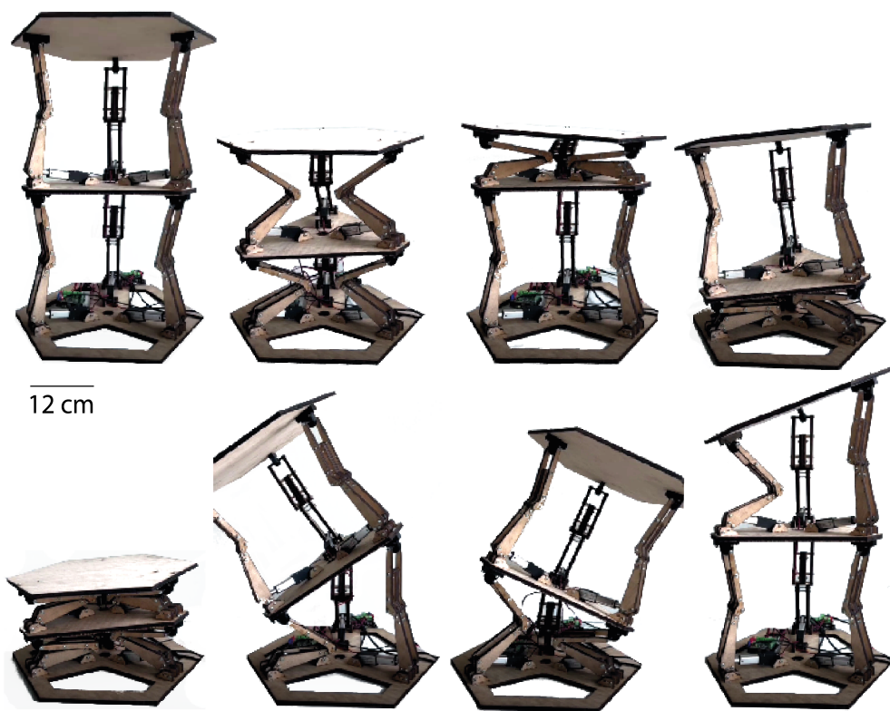
Figure 6.5: Vertical modularity and workspace increase with stacked arm-scale modules. We see how the interaction between neighbour stacked modules is a issue which needs to be tackled to prevent modules to collide.
