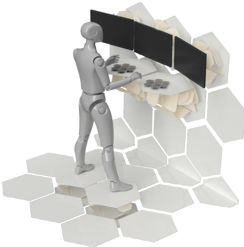
Figure 13.2: Whole-body physically immersive workstation. Human-scale modules on the ground allow whole-body interaction combined with hand-scale modules on the standing desk made of arm-scale modules.
